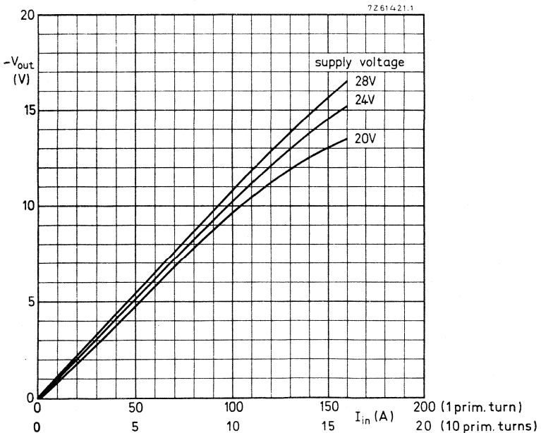
Fig. 2b Variation of d. c. output voltage with d. c. input current.
